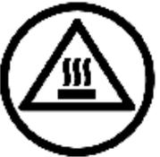
Do not touch the heating elements during operation or after turning off the device, as they may be very hot.
